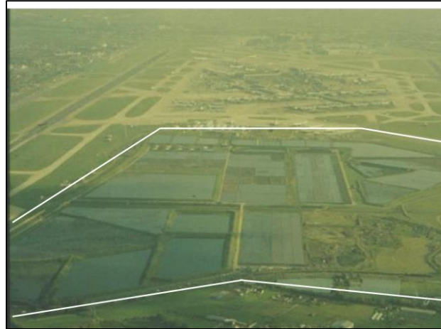
Figure 1: Perry Oaks in the foreground (outlined in white) with the drying beds in the centre, lagoons around the edge and the airport terminals in the background (looking east)
