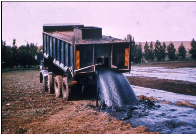
Figure 2: The old sludge application method (ended 1976)
