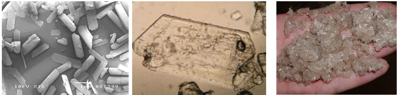
Figure 1: Scanning Electron Microscopy (SEM) and optical microscopy pictures of struvite crystals (left and middle, respectively) and collected struvite (right), adapted from Abma et al. (2010).
