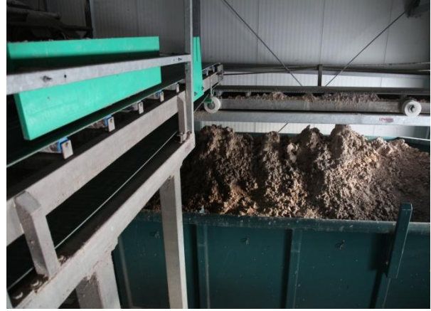
Figure 5: The Phospa TM q and ANAMMOX ® reactors (left) and struvite collection (right) at Olburgen
