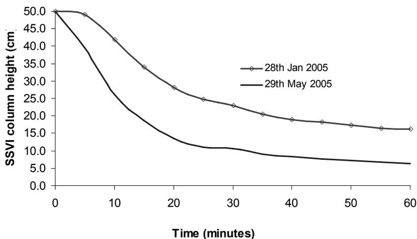
**Figure 2: Zone settling velocities**
