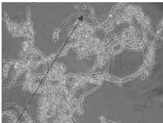
**Figure 4:** January 2005: Type 1851 dominates, Microthrix absent, flocs remain poor (x100)
