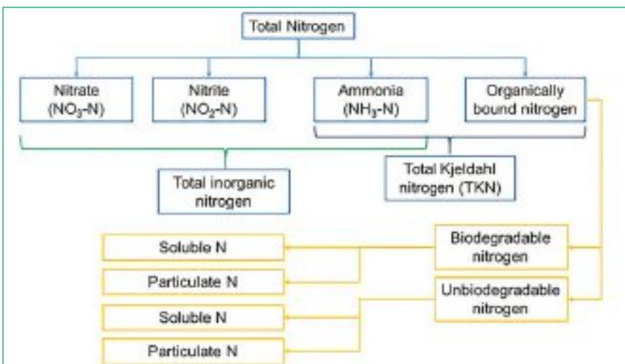
Figure 4. Nitrogen fractionation helps a site to understand how low it can go with discharge levels. The same approach can be adopted for total suspended solids, phosphorus and COD.
