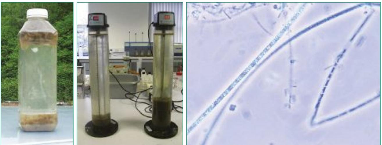
Figure 5. Rising sludge (left) indicative of denitrification or overdosing polymer, the Stirred Sludge Volume Index test (middle) and Thiothrix filament with i) Sulphur inclusions and ii) snapped following hypochlorite dosing.
