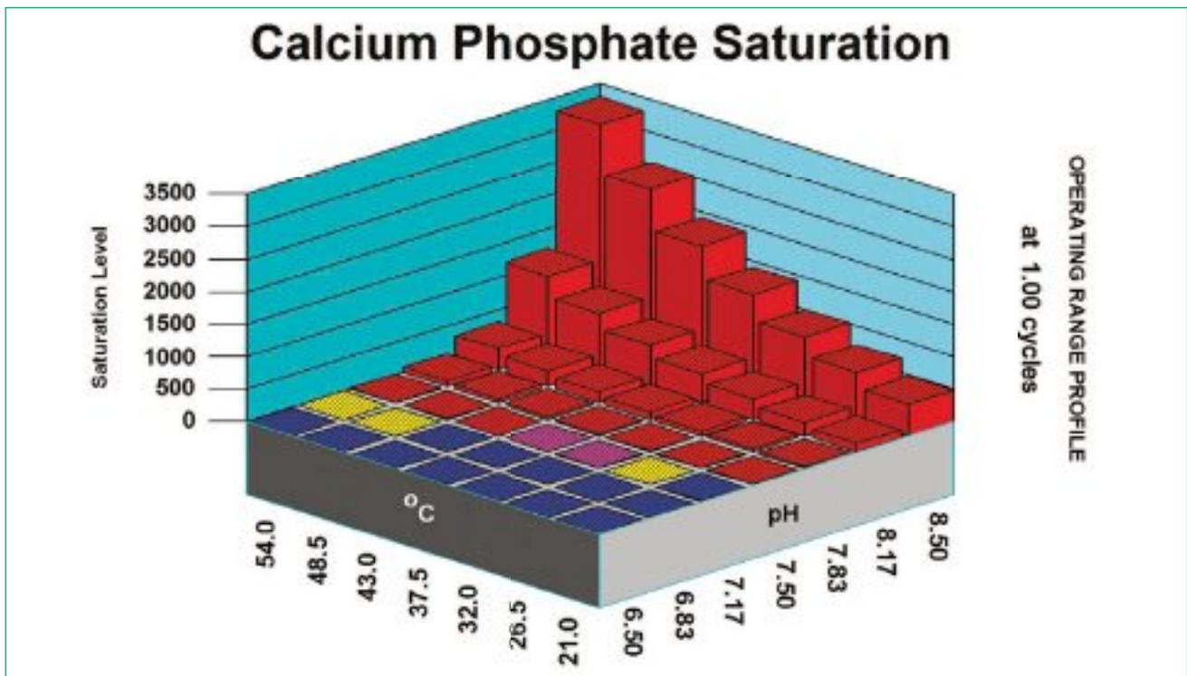
Figure 6. French Creek Analysis output graph illustrating the scale potential of Calcium Phosphate, solubility reduces with increasing temperature and pH. Red warns of a problem, treatment or other remedial action is required. Magenta indicates a problem is likely, take corrective action. Yellow warns to check measurements, trouble is near. Green indicates a mild problem. Blue signifies a safe range.
